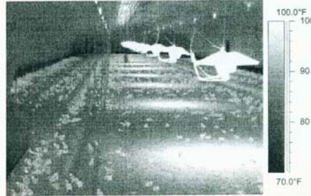
Figure 13. Center house floor temperatures.
