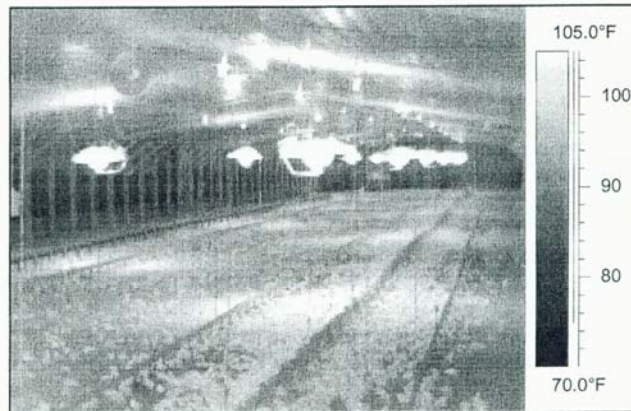
Figure 1. Thermal image of brooding area with radiant brooders.
